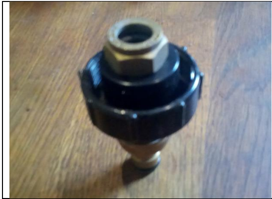
Image 1. Using a 15mm compression nut, without the olive, to secure the union that will take the Hozelock fitting.
