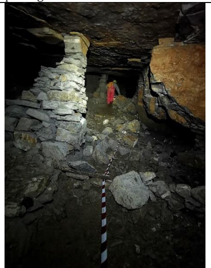
M1 Passage, along the abandoned working face – deeply undercut, and ready to drop.
