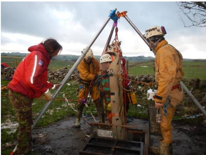
There is no photo from the day, but here is a picture of the Multipod in use on a training exercise at Wharf Engine Shaft, showing how it can lift a vertical stretcher completely clear of the shaft.
